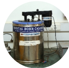
Bomb Calorimeter Bio-diesel property testing
